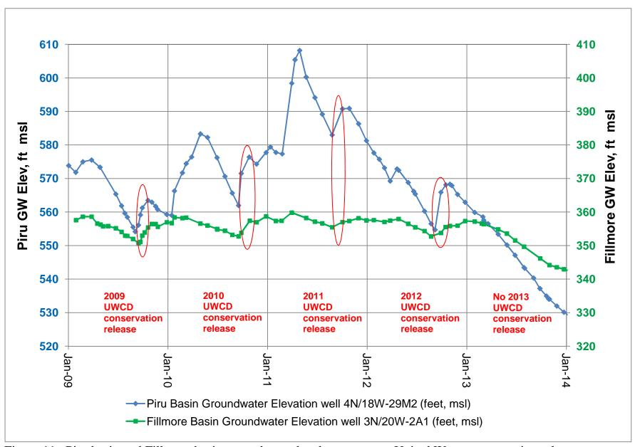
Figure 11. Piru basin and Fillmore basin groundwater levels response to United Water conservation releases.
