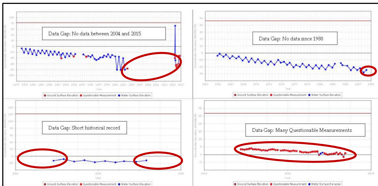
Figure 5-3: Examples of Hydrographs with Temporal Data Gaps (reproduced from DWR BMP #2 - Figure 5, red circling added for clarification).
